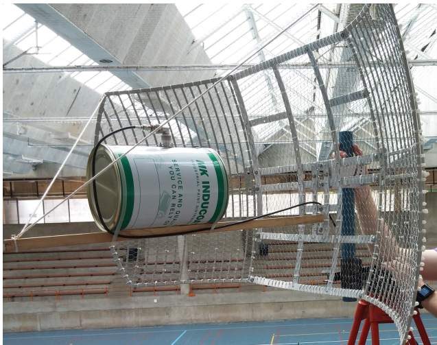
Figure: L-Band antenna prototype with dual polarised circular waveguide feed
