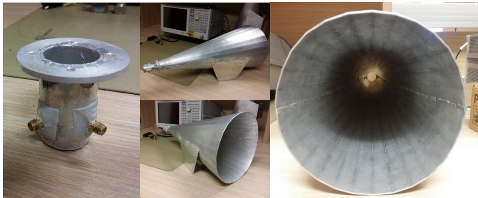
Figure: X-Band conical horn antenna prototype with the dual polarised waveguide feed.
